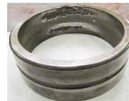
ABOVE: Severely damaged outer race
