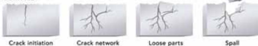
ABOVE: The typical development of a bearing spall
