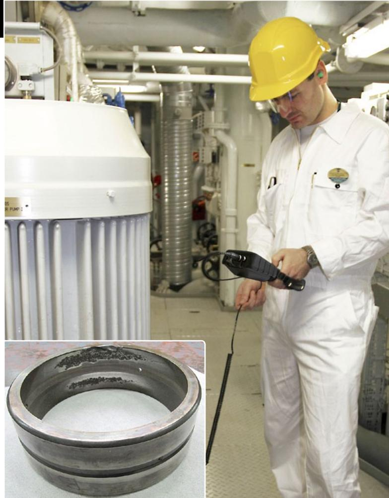
▲ Example of severely damaged outer race. The damage process was monitored for more than a year, enabling the replacement to be planned at the best possible time.
