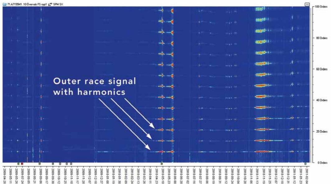
FIGURE 3. This Color Spectrum Overview contains several thousand spectrums spanning over 21 months. The red color indicates fresh spalling, clearly visible in the increasing and decreasing signal pattern typical for this application.
