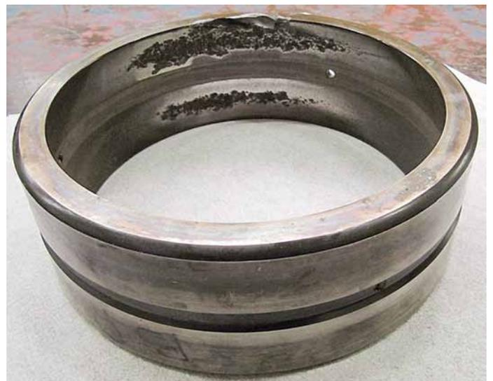
FIGURE 4. Severely damaged outer race of the twin wire press bearing. The damage process was monitored for more than a year, enabling the replacement to be planned at the best possible time.
