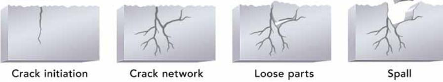
FIGURE 1. A typical bearing spall development pattern.
