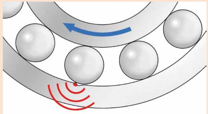
Even well lubricated bearings in mint condition emit very small shocks that can be captured and measured.
